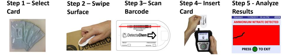
The swipe-card is the key to the flexibility of the Seeker XDU<sup>™</sup>. Each swipe-card contains within it the colorimetric chemistries required for detecting all 5 major groups of explosives. Identification swipe-cards are available for Ammonium Nitrate (AN) and Urea Nitrate (UN).
